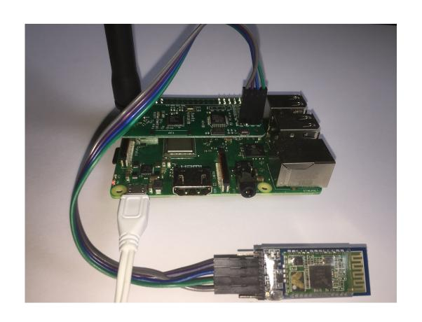
MMDVM GND to HC-05 GND MMDVM TXD to HC-05 RXD MMDVM RXD to HC-05 TXD MMDVM 5V to HC-05 VCC
